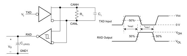
图 20. t<sub>LOOP</sub> Test Circuit and Voltage Waveforms
