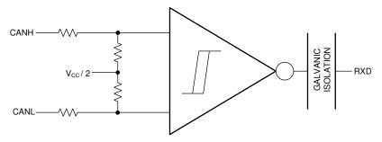
图 26. Simplified Recessive Common Mode Bias and Receiver
