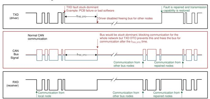
图 27. Example Timing Diagram for TXD DTO
