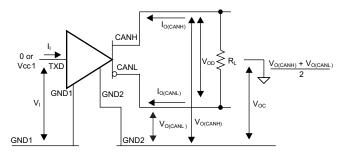
图 15. Driver Voltage, Current and Test Definitions
