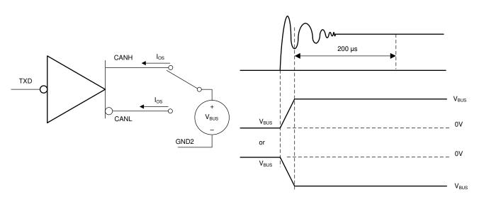
图 23. Driver Short-Circuit Current Test Circuit and Waveforms
