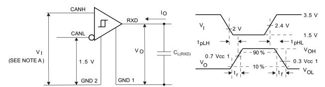
A. The input pulse is supplied by a generator having the following characteristics: PRR  $\leq$  125 kHz, 50% duty cycle,  $t_f \leq$  6 ns,  $t_f \leq$  6 ns,  $t_G =$  50  $\Omega$ .
