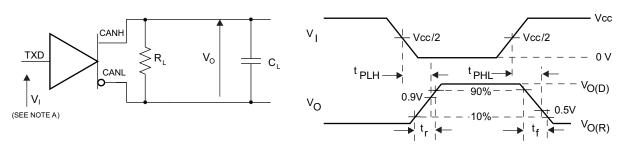
A. The input pulse is supplied by a generator having the following characteristics: PRR  $\leq$  125 kHz, 50% duty cycle,  $t_f \leq$  6 ns,  $t_f \leq$  6 ns,  $Z_O =$  50  $\Omega$ .
