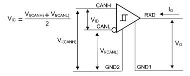
图 18. Receiver Voltage and Current Definitions
