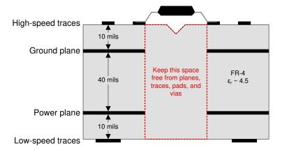
Figure 34. Recommended Layer Stack
