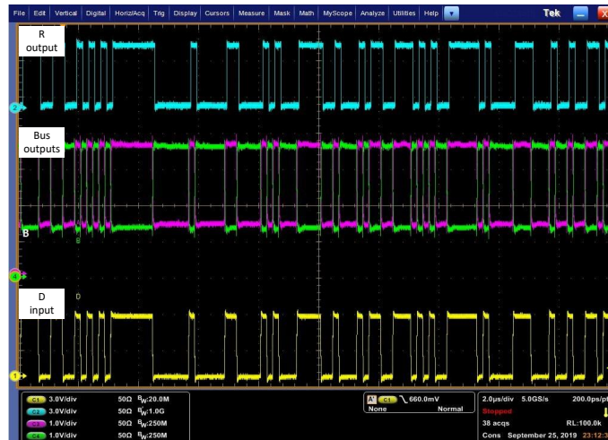
图 22. Waveforms at 10 Mbps Operation, PRBS7 Data Pattern
