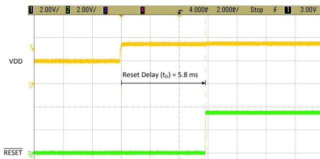
图 54. TPS3840EVM \overline{\text{RESET}} Time Delay ( t_D ) with 0.01- \mu\text{F} Capacitor
