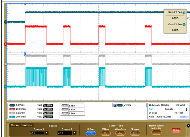
Figure 42. Overcurrent (OCP) Detection
