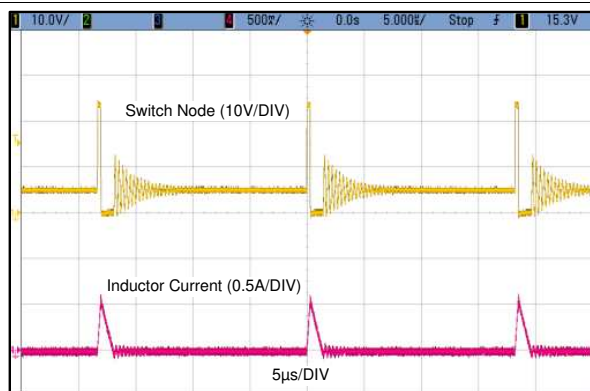
图 9. Typical PFM Switching Waveforms V_{IN} = 24\text{ V} , V_{OUT} = 5\text{ V} , I_{OUT} = 50\text{ mA}
