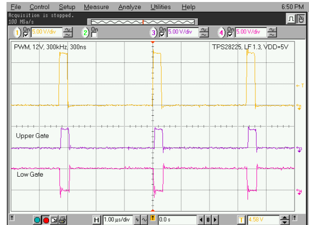
图 6-5. 12-V PWM Pulse at V_{DD} = 5\text{ V}
