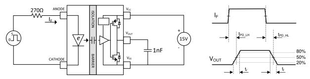
图 7-1. I<sub>F</sub> to V<sub>OUT</sub> Propagation Delay, Rise Time and Fall Time
