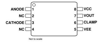
图 5-2. UCC23514M DWV Package 8-pin SOIC-WB Top View
