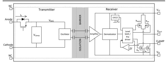
图 8-2. Functional Block Diagram for UCC23514M (Miller clamp)
