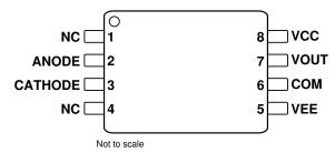
图 5-1. UCC23514E DWV Package 8-pin SOIC-WB Top View
