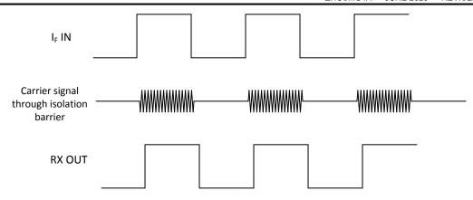
图 8-5. On-Off Keying (OOK) Based Modulation Scheme
