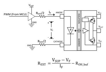
图 9-6. Configuration 2: Driving the input stage of UCC23514 with one Buffer and split resistors
