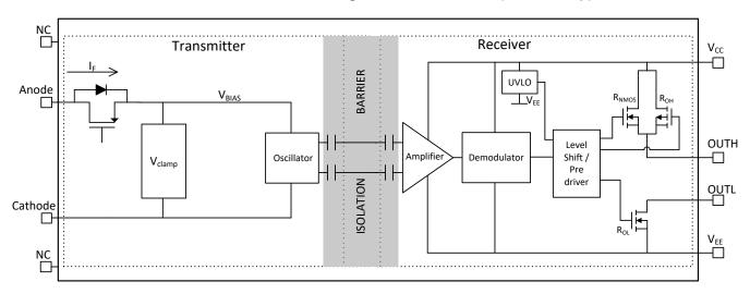
图 8-3. Functional Block Diagram for UCC23514S (Split output)
