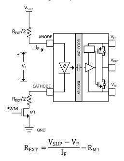
图 9-5. Configuration 1: Driving the input stage of UCC23514 with a single NMOS and split resistors
