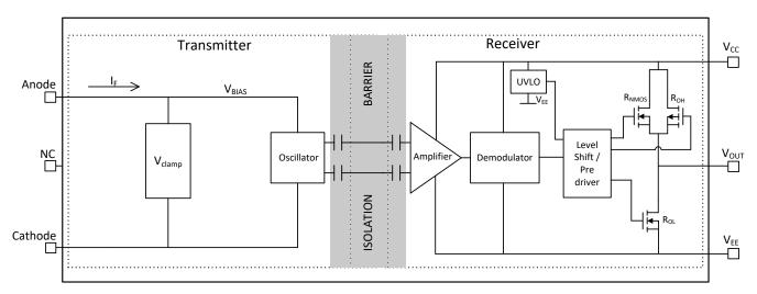
图 8-4. Functional Block Diagram for UCC23514V (single output pin)
