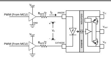
$$R_{EXT} = \frac{V_{SUP} - V_F}{I_F} - (R_{OH\_buf} + R_{OL\_buf})$$
