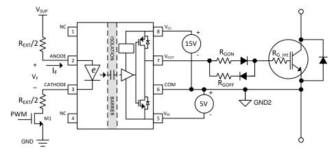
图 9-1. Typical Application Circuit for UCC23514E to Drive IGBT with Split Gate Drive Supply
