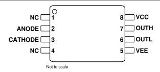
图 5-3. UCC23514S DWV Package 8-pin SOIC-WB Top View
