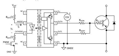
图 9-3. Typical Application Circuit for UCC23514S to Drive IGBT
