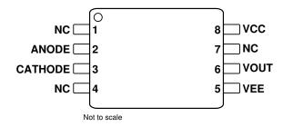
图 5-4. UCC23514V DWV Package 8-pin SOIC-WB Top View
