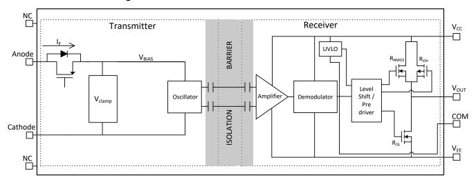
图 8-1. Functional Block Diagram for UCC23514E (COM pin connection to IGBT Emitter)
