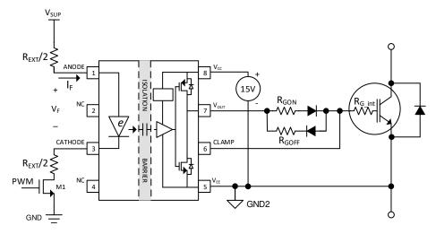
图 9-2. Typical Application Circuit for UCC23514M to Drive IGBT
